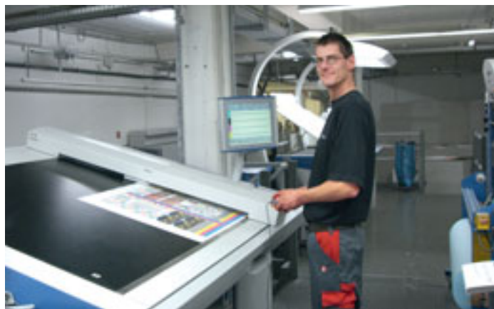
Thomas Bleek measuring the colour densities on the Rapida 142 using a DensiTronic 5 closed-loop colorimetry system
