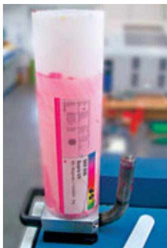
The ink ducts are automatically filled with ink from cartridges
