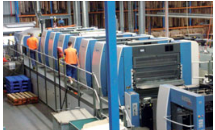
The Rapida 142 seven-colour coater press with extended delivery at Glama Pak is mounted on a 210mm (8 1 / 4 in) plinth so that it can handle higher piles
