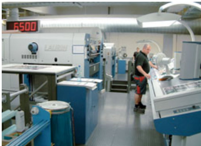
Schur Pack's three Rapida 142 large-format presses (pictured here) and Rapida 105 eight-unit medium-format press all comply with the specifications laid down by ISO 12647-2. The Rapidas each bear individual names on the drive side
