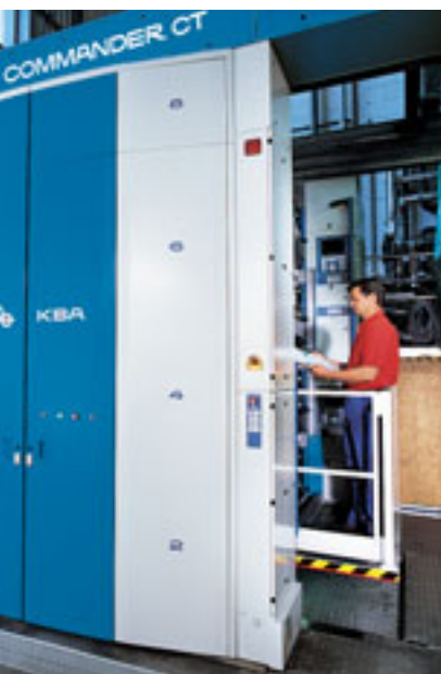
Ergonomic lifts at the Commander CT tower mean that operators no longer have to climb stairs or walk long distances
