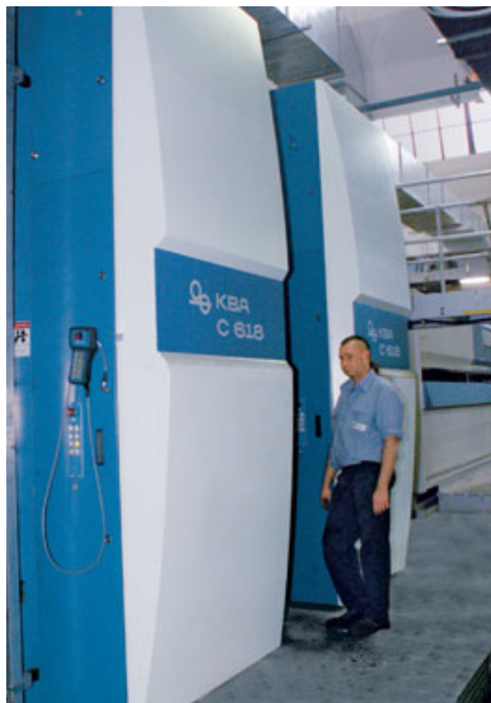
The Compacta 618's massive printing units can deliver 2 x 72 book pages measuring 190 x 240mm (7½ x 9½in) in one or two colours
