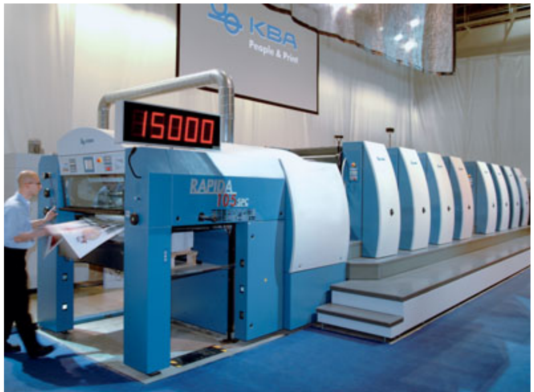
What a stunning performance: four perfecting jobs of 500 sheets apiece entailing three plate changes plus a change of format and substrate (with conversion of perfecting unit and automatic suction-ring positioning) were printed in just under 24 minutes on an eight-colour Rapida 105 featuring DriveTronic SPC direct drives
