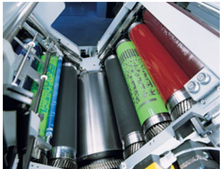
The Genius 52UV's keyless inking units, which have just one anilox roller and a forme roller, can be cleaned quickly and easily
