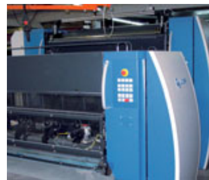
The Rapida 162 at Sittic has five printing units, automatic plate changers, a coater and a hybrid capability for inline coating
