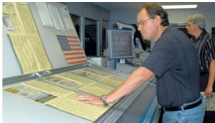
One of the two ErgoTronic control consoles for the Compacta 818 is located behind the folder. Press controls include ColorTronic ink-key setting desks, a LogoTronic Basic presetting system and a colour and cut-off register system
