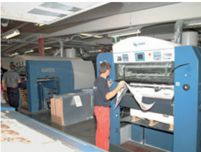
The ten-colour (in the background) and eight-colour Rapida 105 perfecter presses at Swedish print enterprise Strokirk Landströms have DriveTronic SPC direct plate-cylinder drives which deliver a high level of productivity despite frequent job changes
