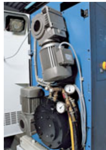
On the Rapida105 with DriveTronic SPC the plate cylinders are driven directly by high-torque motors which are synchronised electronically with the utmost precision and supersede the gears and couplings used in conventional drive systems
