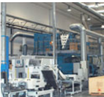
The Compacta 215 can deliver copies via an F3 gripper folder or a Vits-Rotocut sheeter (left front)
