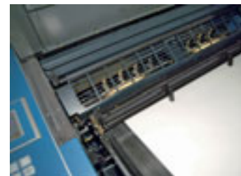
The long Rapida 105 at Leo Koitzsch's nine-employee printing company incorporates a DriveTronic SIS no-sidelay infeed system
