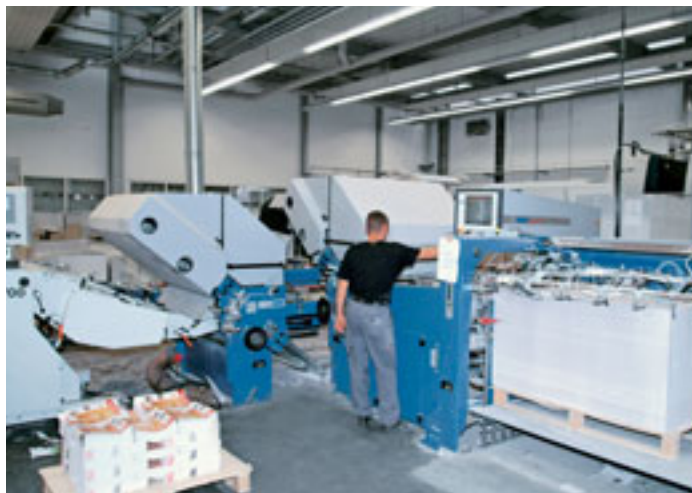
A large-format MBO folding machine has been installed in the finishing department, but the Rapida 142's high output will soon make it necessary to install a second one
