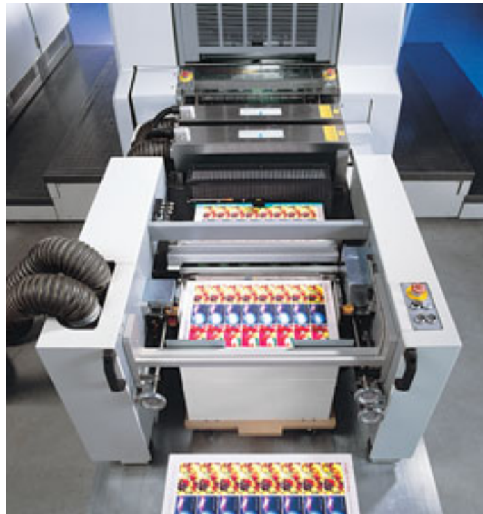
The Genius 52UV's extended delivery has an integrated UV dryer
