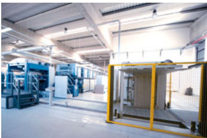
The Rapida 162a at Eurografica is embedded in an automatic pile logistics systems
