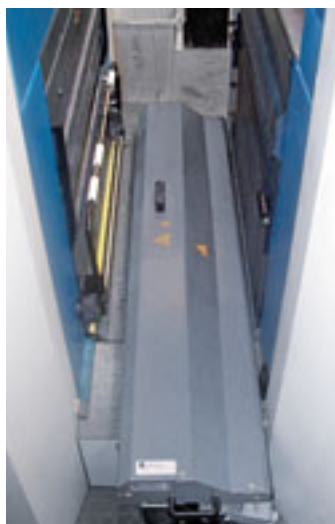
An UV dryer after the first printing unit ensures that the inks and coatings subsequently applied can adhere firmly to the substrate
