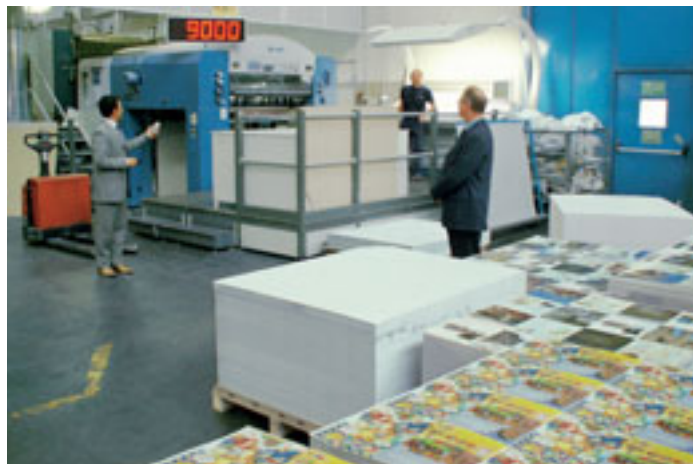
Rotolito Lombarda prints 4/4 books on medium- and large-format KBA Rapida sheetfed offset presses
