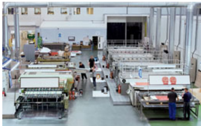
Screen printing presses, one of them (on the right) a Thieme 5070, operate alongside the two Rapida 205s at Capital
