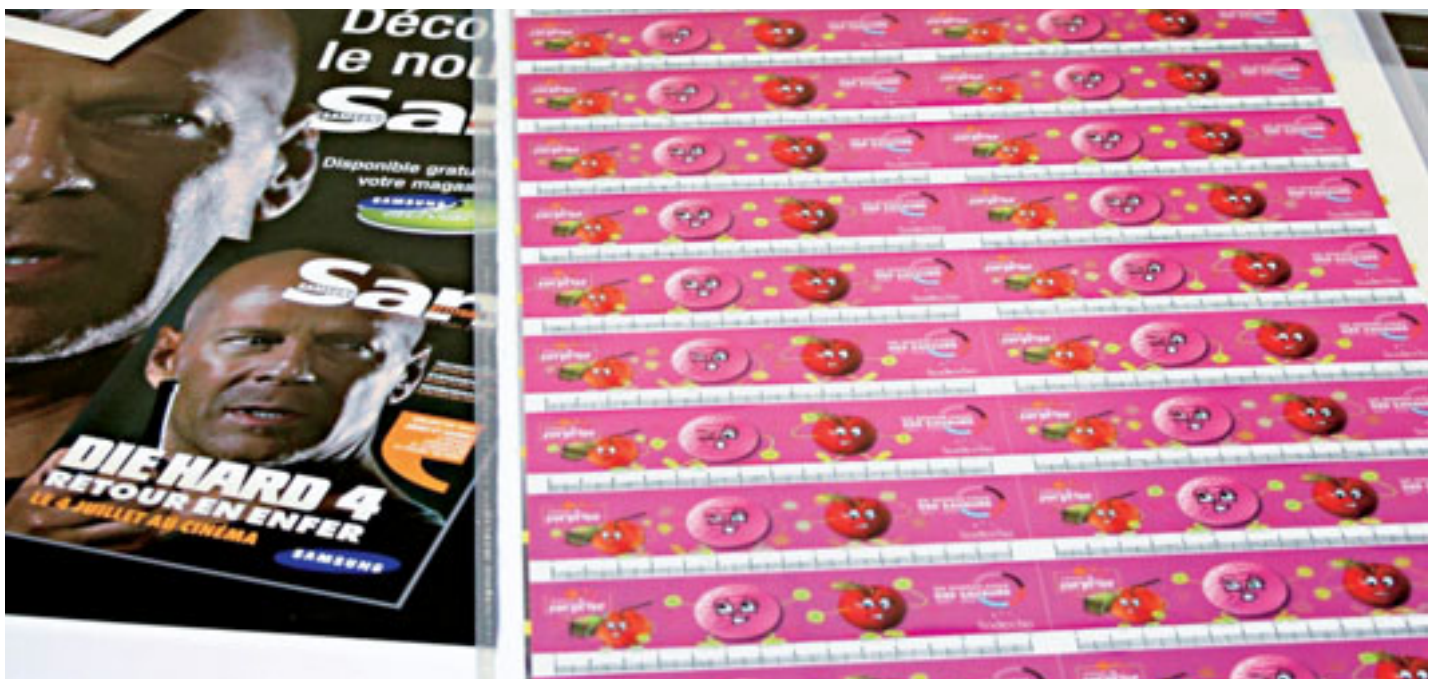
Rulers printed on lenticular film in the Genius 52UV. Tilting them back and forth makes the ice-cream scoops jump up and down and laugh
