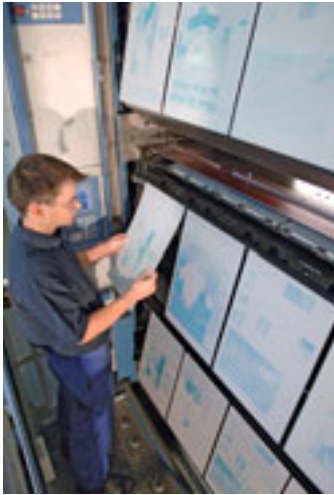
The Commander CT, like the Cortina, is available with PlateTronic systems for automatic, on-the-fly plate loading and disposal in just two minutes, irrespective of the number of plates
