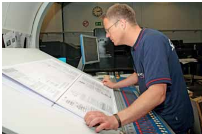
Even though quality monitoring with QualiTronic colour control eliminates the need for adjustments at the ink keys, Michael Dörpinghaus still checks the sheets out of sheer habit
