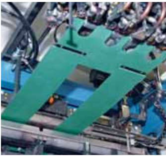
Fleece-covered sheet guide in the DriveTronic feeder
