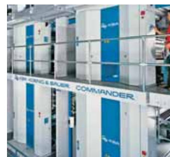
The stacked nine-cylinder satellites deliver a top-quality print and allow straightforward 4/4 production, which will not be confined solely to newspapers
