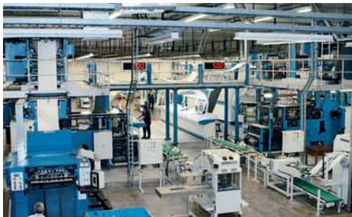
The webs of the two presses can be guided over a transverse link to a single folder
