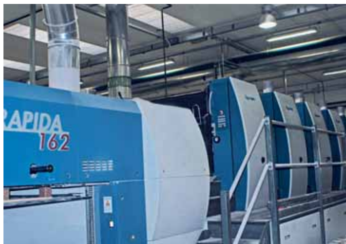
The five-colour Rapida 162a installed in mid-2008 is D'Auria's fourth KBA sheetfed press since 1998
