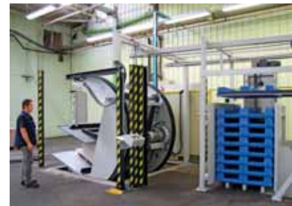
An automated pallet preparation system (pictured) and automated pallet logistics allow the Rapida 142's nonstop capabilities to be exploited to the full
