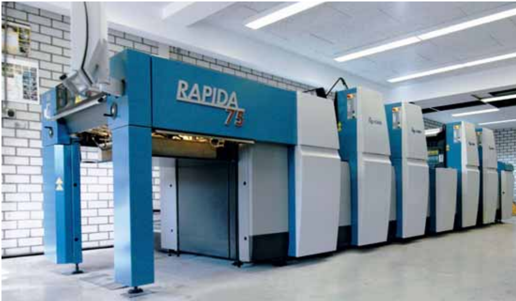
Vis Offset's Rapida 75 four-colour press with automatically convertible perfecting after the second unit
