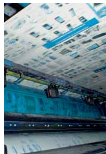
Even with a narrower web width of 1,680mm the Compacta 818 can print 64pp copies measuring 210 x 299mm untrimmed in addition to 48pp and 56pp copies
