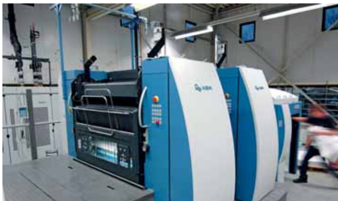
During a flying job change the plates are changed in one pair of printing units (1 plus 3 or 2 plus 4) while mono perfecting takes place in the other pair
