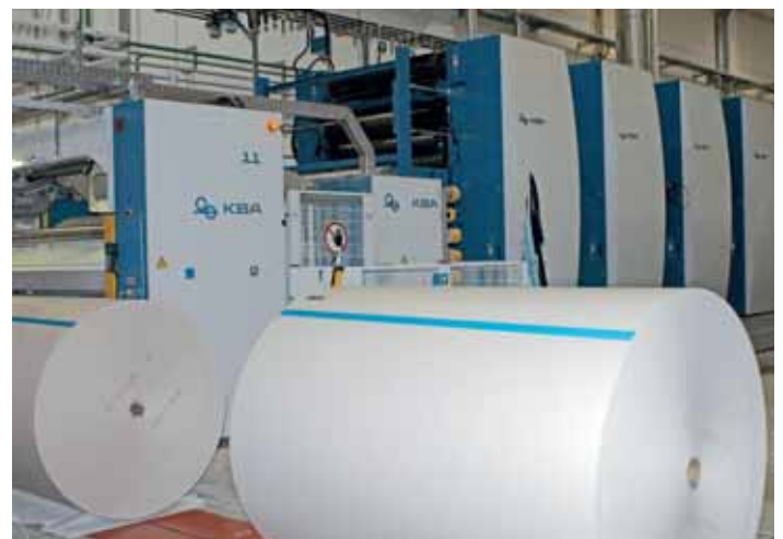
The Compacta 215 installed in 2006 is also embedded in the KBA Patras A automated reel-logistics system
