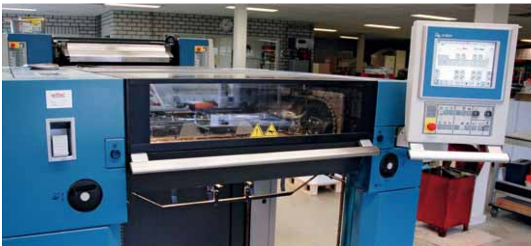
A touch-screen (right) at sheet delivery allows rapid intervention
