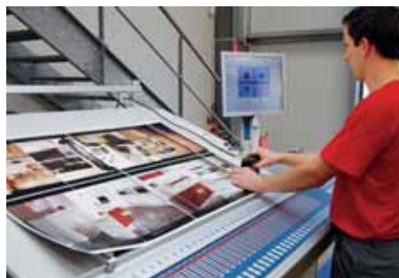
Automatic register setting with ErgoTronic ACR (video magnifier) is simple and reliable
