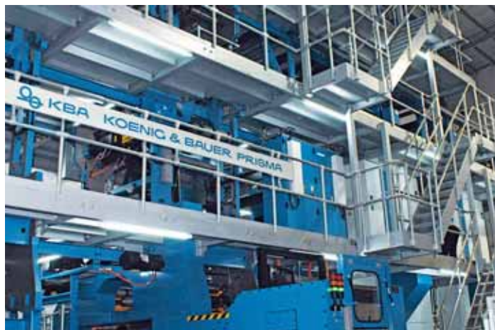
The Prisma in Ahmedabad, with its nine four-high towers, nine reelstands, one double and one single folder, has a formidable production capacity
