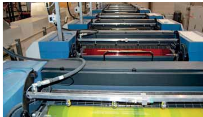
All the inks consumed at Impression Rochelaise are based on vegetable oils, and the quick response inking units are connected to a central pumping system
