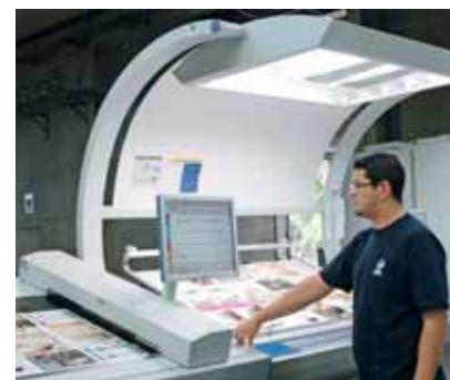
The controls for the new KBA sheetfed presses include a DensITronic Professional closed-loop densitometric colour measurement and control system to the left of the ErgoTronic console
