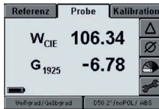
Measuring CIE whiteness and ASTM yellowness with Techkon's SpectroDens Premium (0°/45°)
