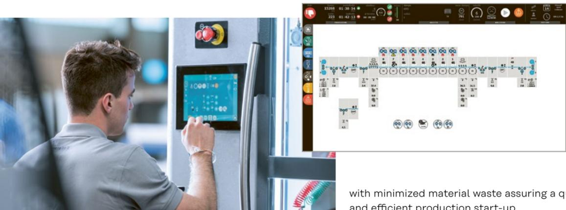
**ErgoTronic** is the name of the new control system for Koenig & Bauer Flexotecnica printing presses featuring completely new PLCs, motion logic drives and high quality industrial operator panels to achieve increased system performance, accuracy and reliability.
