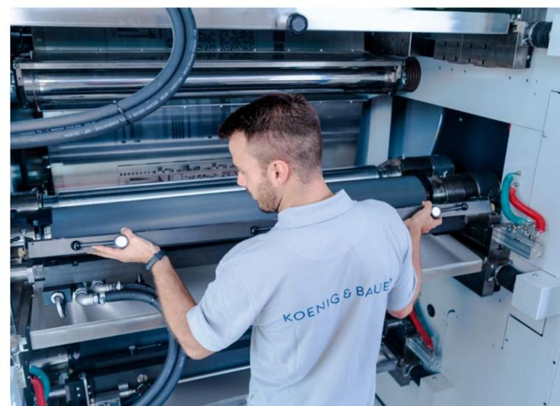
New doctor blade chamber with innovative design by Koenig & Bauer Flexotecnica
