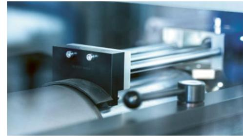
**Pneumatic ejectors** for quick and simple printing and anilox sleeve removal in utmost safety by avoiding scratches or damage, particularly with wide printing widths and large print repeats
