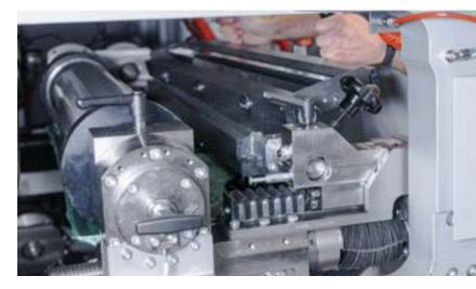
System for quick removal of doctor blade chamber
