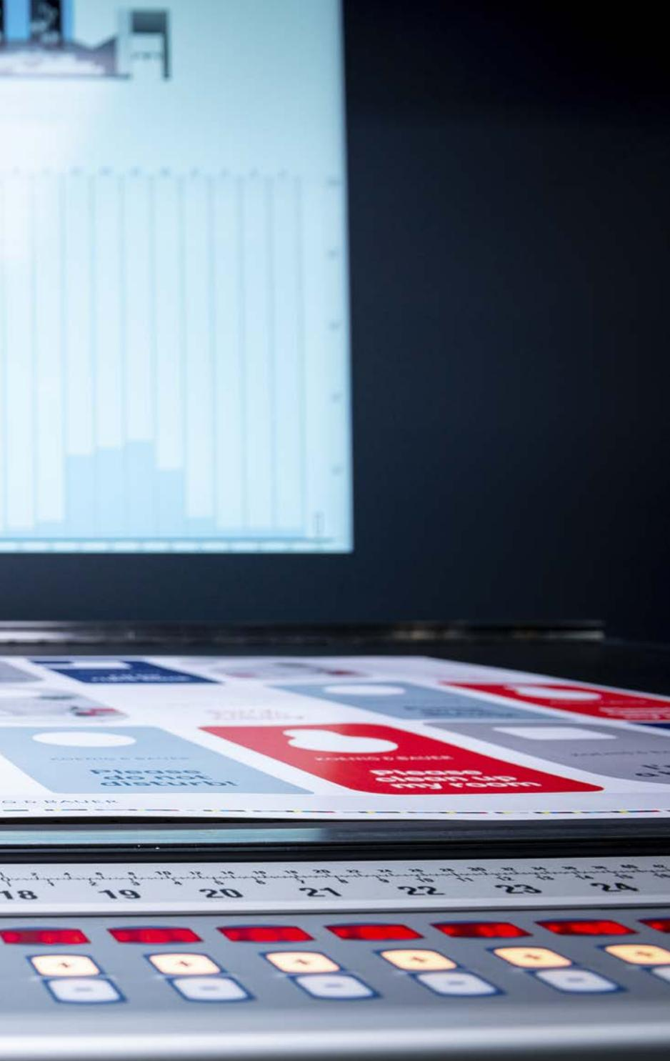
For **register measurement and control**, you can choose between the especially compact solution ErgoTronic ACR and the automatic system ErgoTronic ICR. In both cases, necessary corrections are calculated for the lateral, circumferential and diagonal register settings.
