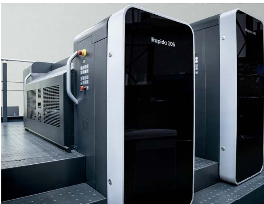
The same extensive flexibility applies with regard to the potential fields of application for the Rapida 105: for **commercial printing**, the press can be supplied in configurations with up to eight inking units and facilities for 4-over-4 perfecting in an inline process.
