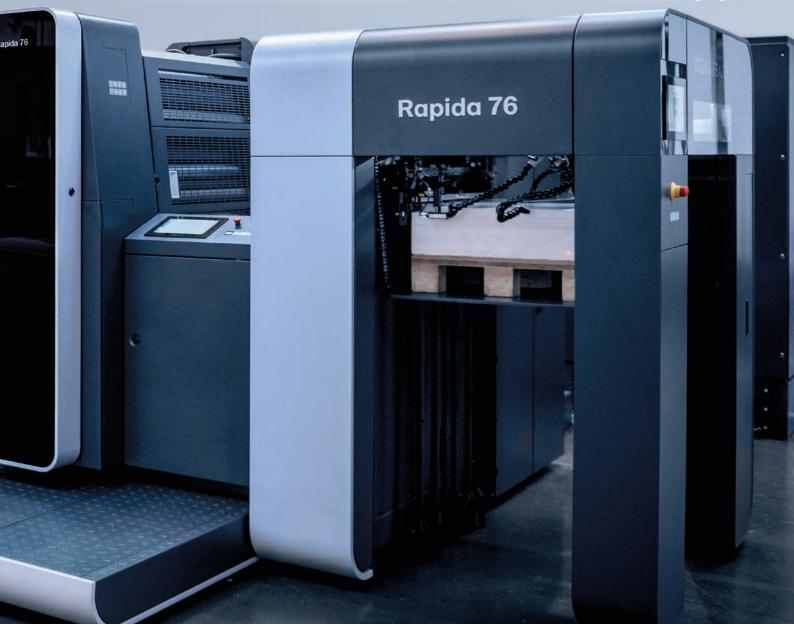
Packaging printers benefit from **application-oriented configurations** with up to eleven printing and finishing units. Equipment packages extend the already wide range of substrates to include heavier boards or plastic films.
