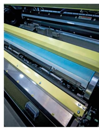
to apply and later wash down roller oil. As a further benefit, an inking unit currently not in use can also be prepared for the next job while the current production continues.
