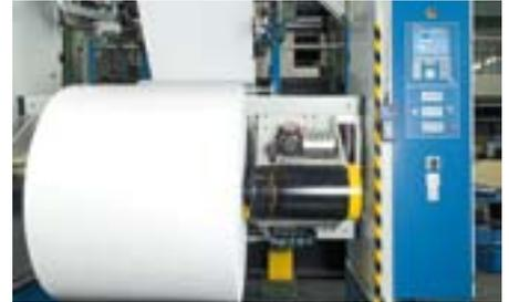
The reels are braked and driven by low-maintenance AC drives located in the reelstand arms
