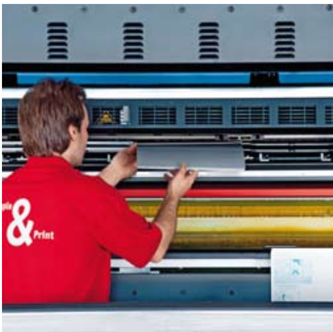
Our intelligent PlateTronic plate-changing system slashes edition changes by allowing the feed magazines for the plates to be loaded and emptied while the press is up and running
