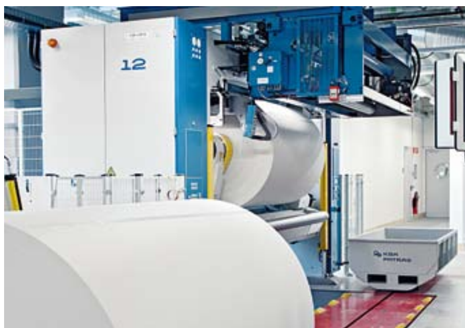
Right: Automated reel logistics from splice preparation to the AGV-accessed reel store and the reelstand
