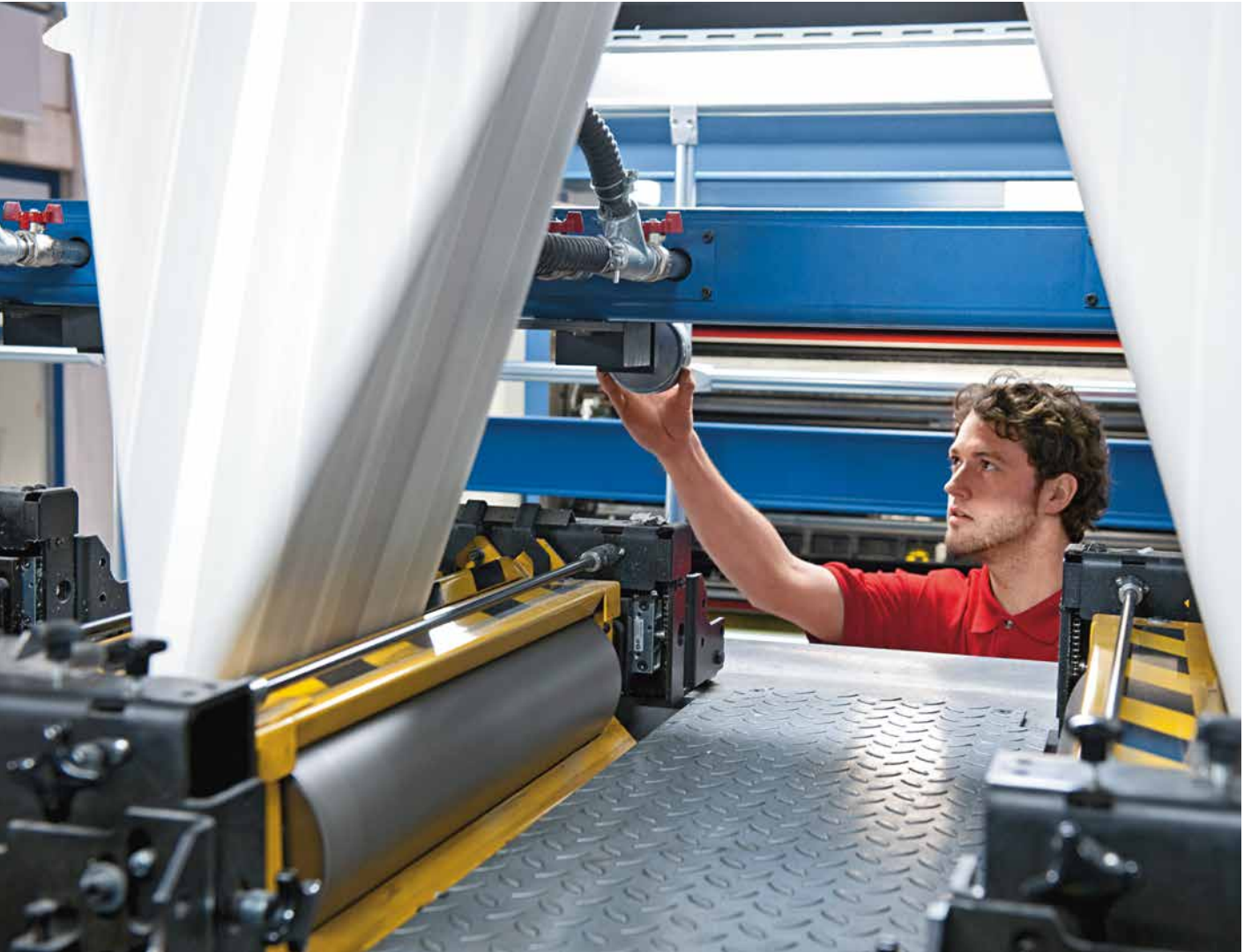
An automatic chain web-up system on the drive side of the press accelerates production preparation
