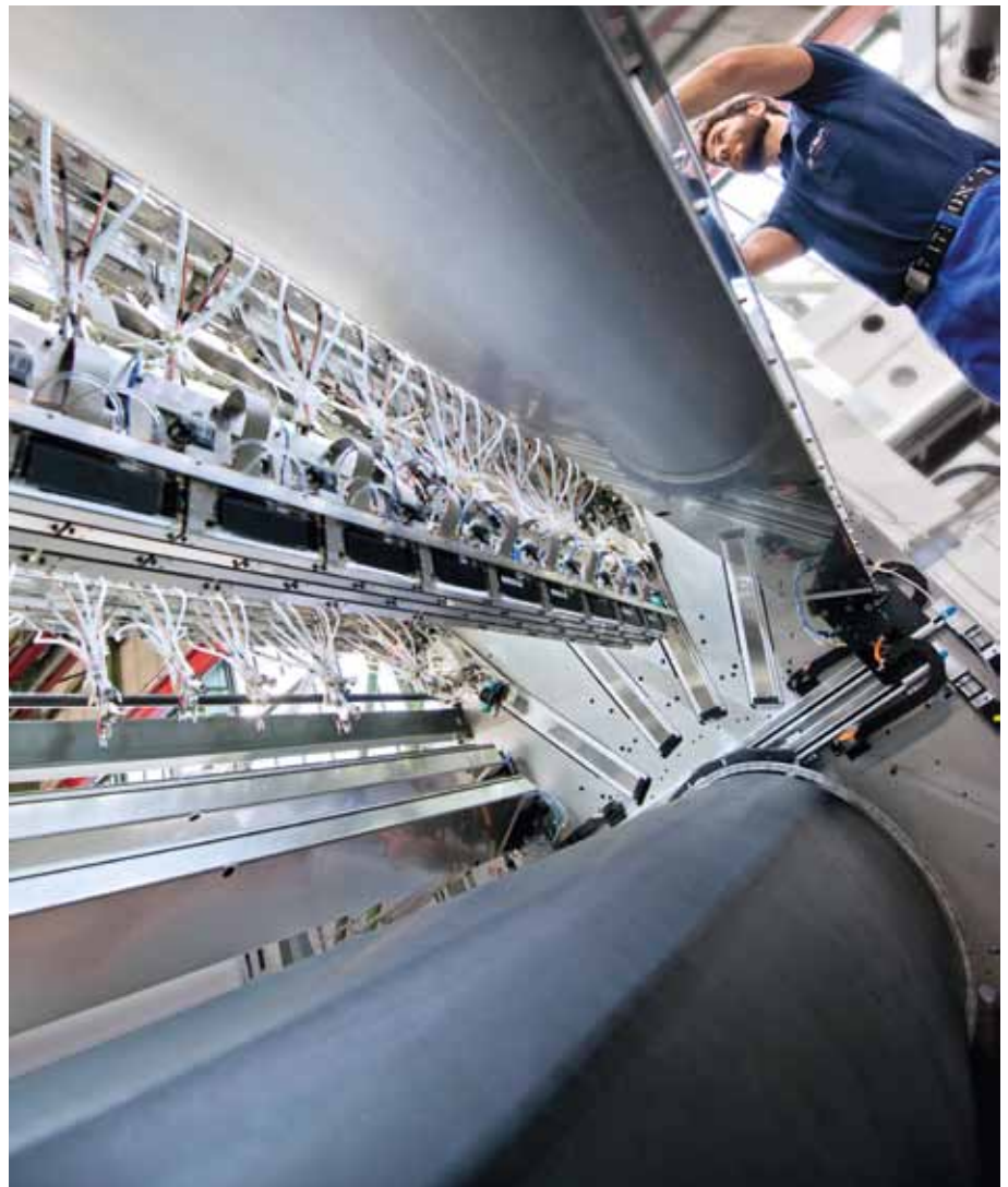
The substrate is guided around the central cylinder and under the printing heads
