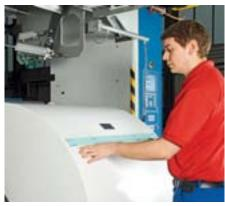
Automatic reelstand that splices precisely at maximum press speed
