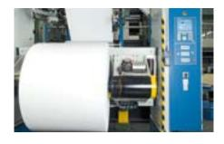
The reels are braked and driven by low-maintenance AC drives located in the reelstand arms
