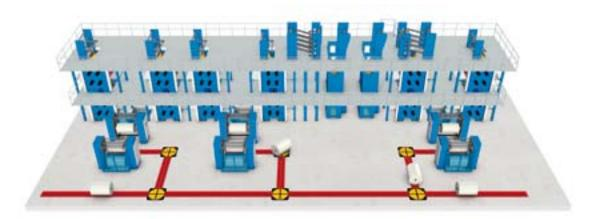
A reelstand positioned at a 90° angle to the press line and embedded in a Patras M manual logistics system
