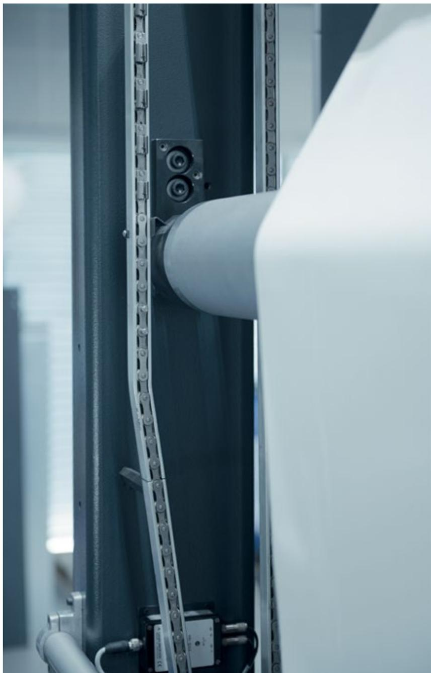
**With its standard features such as fully automatic webbing up with a chain, Koenig & Bauer is linking high-performance features from its offset range of presses with the variability and flexibility of digital printing**
