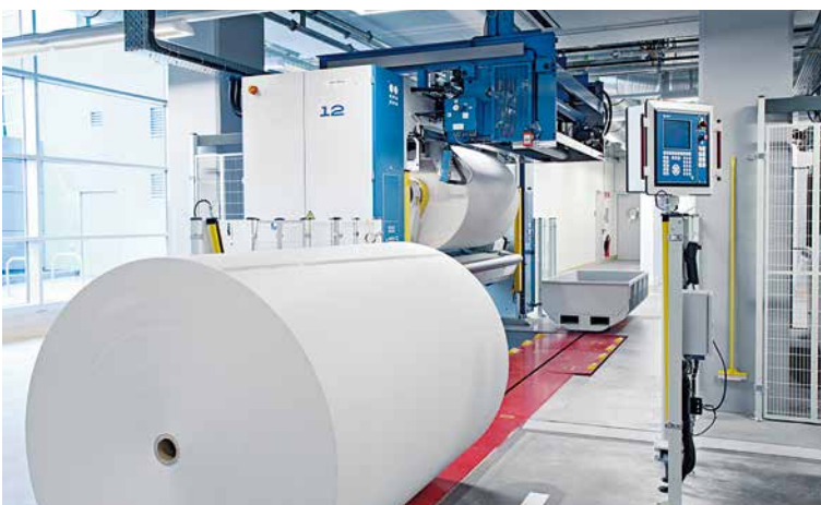
The high-performance Pastomat CL 60 reelstand for reel diameters of up to 1,524mm (60in)
