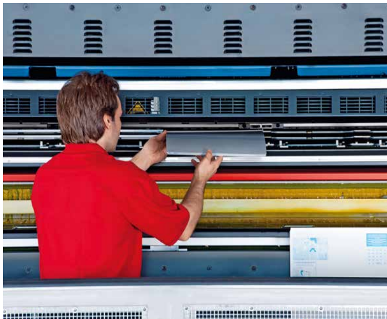
The intelligent PlateTronic plate-changing system slashes edition changes by allowing the feed magazines for the plates to be loaded and emptied while the press is up and running. It is also available for the Cortina
