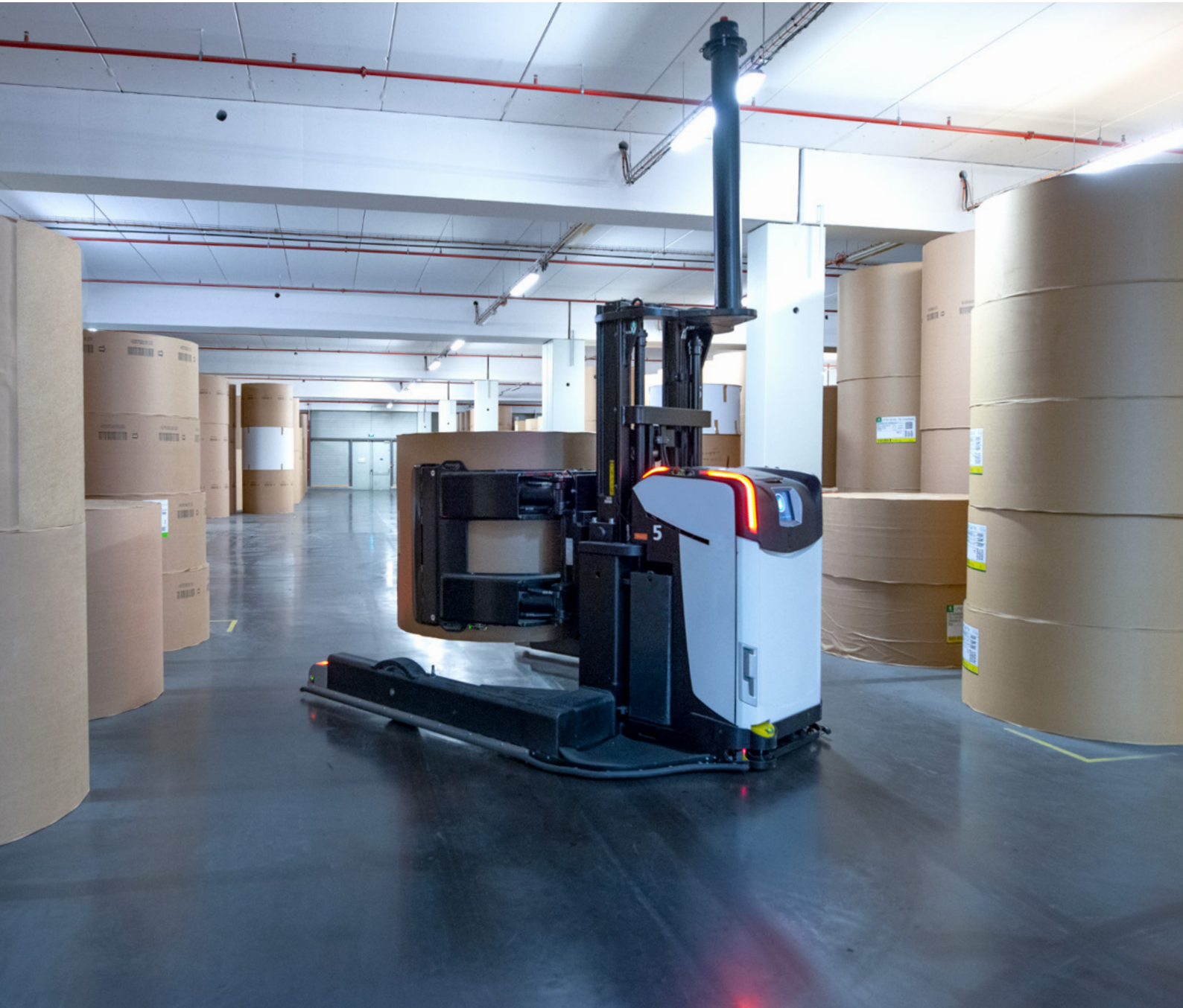
Automated reel transport with computer-controlled clamp AGVs
