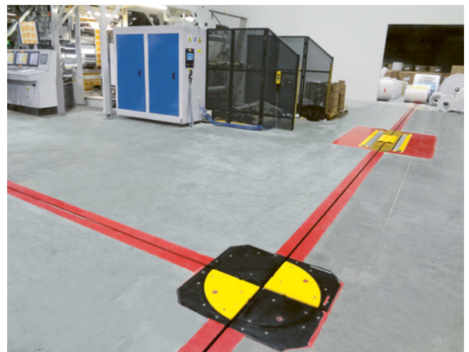
Patras M on two CI flexo presses with stations to unstrip the unprinted reels and pack the finished printed ones.
