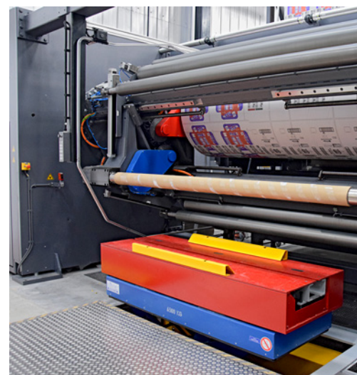
The printed reels are automatically transported from the rewinder to the main store
