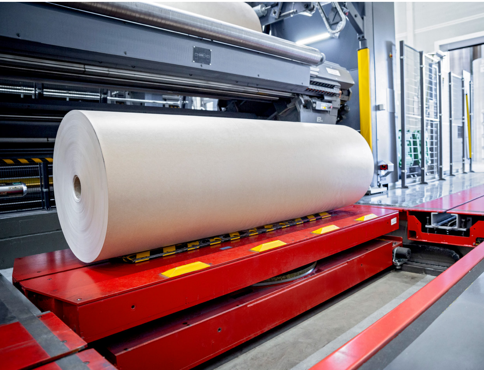
Automatic supply to unwinders, also for particularly wide reels
